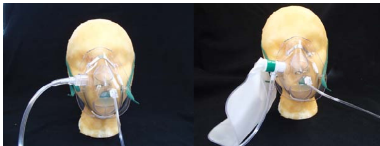
Figure 2 showing a picture of the set ups used during testing. The medium concentration adapter configuration is showed on the left, the high concentration adapter configuration is showed on the right.
